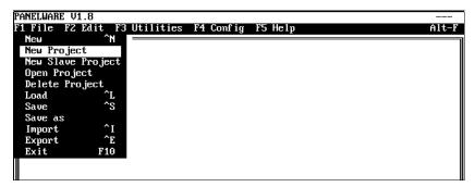
When the **New Project** option is highlighted inversely within the menu, press  $\downarrow$  to open the **New Project** window, in which the project name and the type of Panel Controller to be used are entered.
